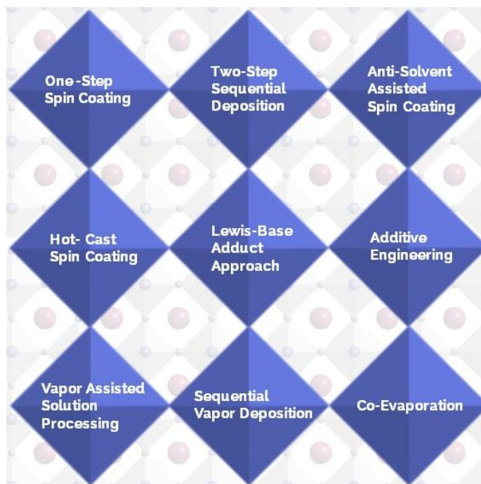
Figure 2. Various methods of growing polycrystalline hybrid perovskite films. [12-13,35-42]
