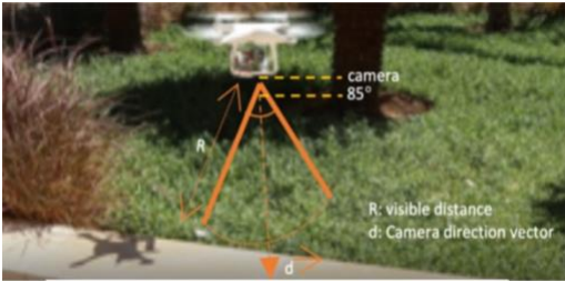
Fig. 6. The camera attached to the drone
