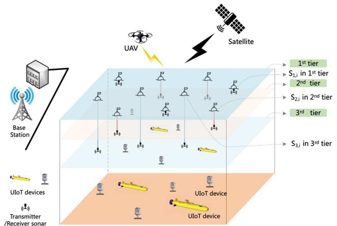
Fig. 1: A diagram of underwater acoustic  $K$ -tier network.
