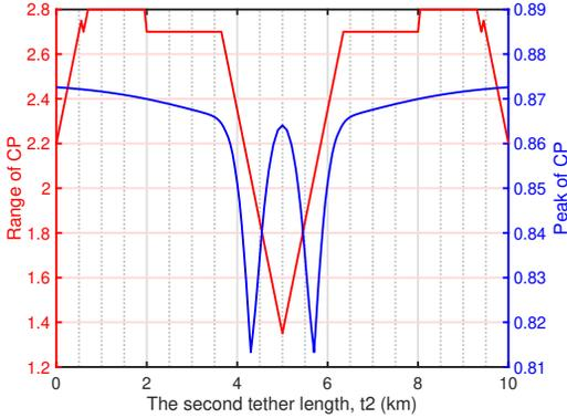
Fig. 7: CP of the two-tier network,  $\gamma_1 = \gamma_2=1$  SSs/km<sup>2</sup>,  $\tau=0.2$ .
