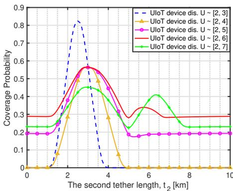
Fig. 8: Range and Peak of CP in a two-tier network with  $t_1=5$  km,  $\gamma_1 = \gamma_2=1$  SSs/km<sup>2</sup>,  $\tau=0.2$  and different distributions of UIoT device's depth.
