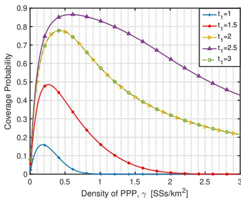
Fig. 4: Range and Peak of CP in single-tier network with different densities of PPPs with  $\gamma=2$  SSS /km<sup>2</sup>.
