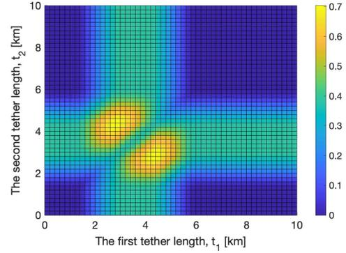
Fig. 9: Optimal two tether lengths in the two-tier network with  $\gamma_1 = \gamma_2=1$  SSs/km<sup>2</sup>,  $\tau=0.2$  and the distribution of UIoT device's depth is  $U \sim [2,5]$  km.
