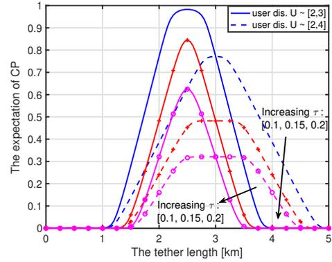
Fig. 5: Range and Peak of CP in single-tier network with the distribution of UIoT device's depth are  $U \sim [2, 3]$  km (solid lines) and  $U \sim [2, 4]$  km (dashed lines),  $\gamma = 2$  SSS/km<sup>2</sup>.
