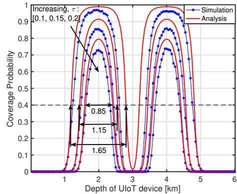
Fig. 6: CP of the two-tier network, under the situation that  $\gamma_1 = \gamma_2 = 2$  SSS/km<sup>2</sup>,  $t_1 = 2$  km,  $t_2 = 4$  km.
