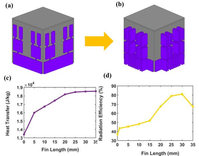
Fig. 1. (a) 2D flat antenna with three Cantor fractal iterations (b) Heatsink antenna (c) Heat transfer rate as a function of fin length (d) Antenna radiation efficiency as a function of fin length
