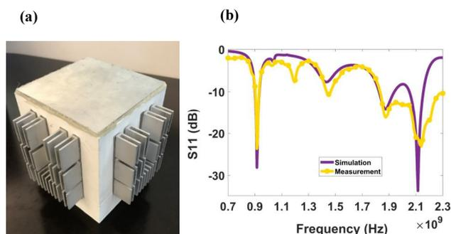
Fig. 2. (a) Fabricated heatsink antenna assembled on the body of the thermal energy harvester (TEH) (b) Reflection coefficient of the heatsink antenna
