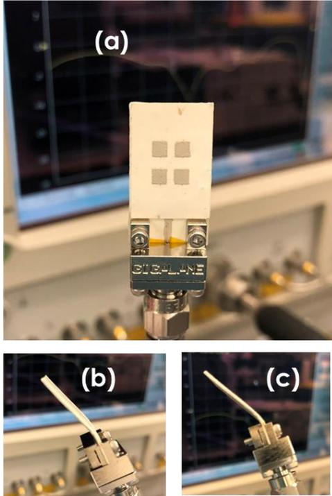
Fig. 10. Measurement setup (a) flat, (b) low bending i.e. Bend\_1 and (c) moderate bending i.e. Bend\_2 condition.
