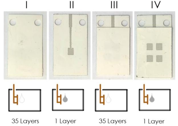
Fig. 8. Fabrication steps for the antenna design.
