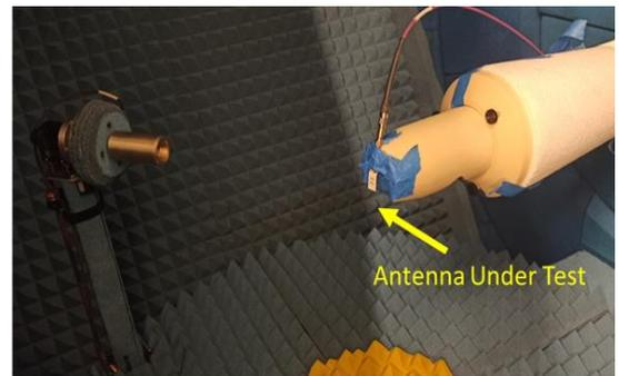
Fig. 13. Antenna radiation pattern measurement setup.
