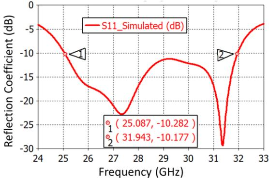
Fig. 6. Simulated reflection coefficient of the antenna
