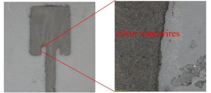
Fig. 9. Microscopic images of the fabricated driven patch using the screen printing.
