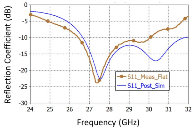
Fig. 12. Comparison of measured and post-simulation reflection coefficients.
