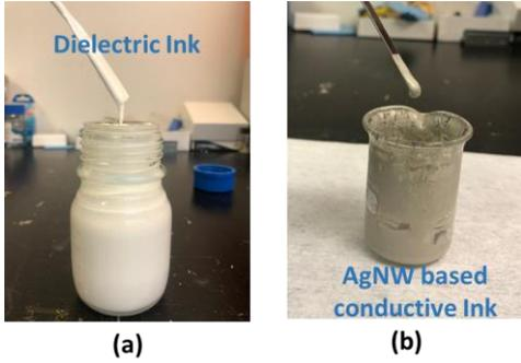
Fig. 1. Screen printable (a) dielectric ink and (b) AgNW based conductive ink
