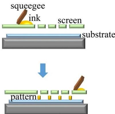
Fig. 3. The standard screen printing process
