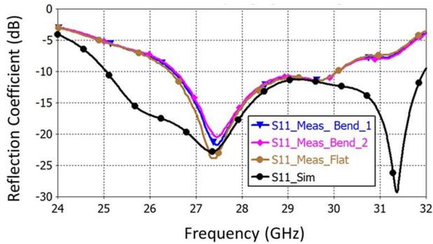
Fig. 11. Measured reflection coefficient for flat and various bending conditions plotted against simulated reflection coefficient in a flat condition.
