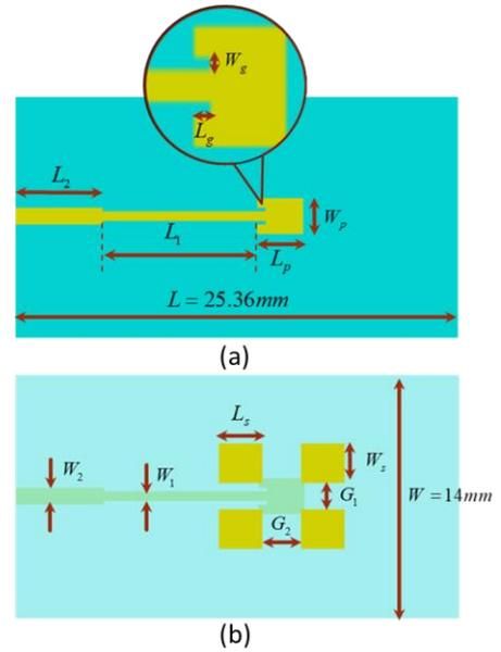
Fig. 5. Detailed design description of the antenna (a) driven patch layer, and (b) superstrate top layer.
