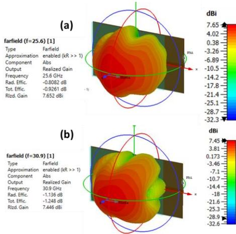
Fig. 7. The simulated 3D radiation pattern of the antenna at (a) 25.6 GHz and, (b) 30.9 GHz.
