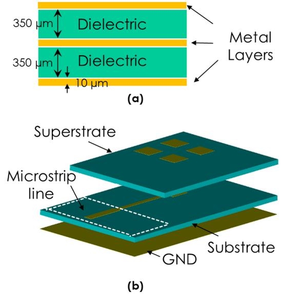
Fig. 4. (a) Antenna stack-up (b) exploded view of antenna layers.
