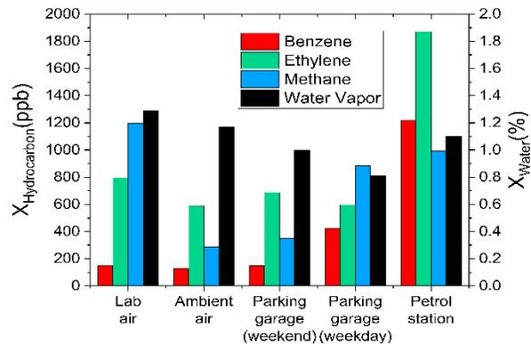
Fig. 3. Measured concentrations of benzene, ethylene, methane and water vapor in the collected samples
