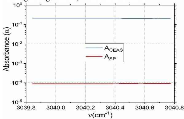
Fig. 2. Comparison of CEAS absorbance with simulated single-pass absorbance (X = 165 ppb, T = 298 K, P = 1 atm, L = 50 cm)
