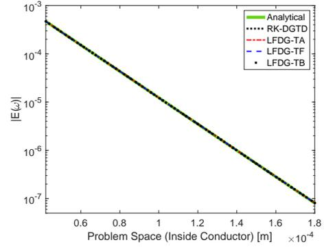
Fig. 3. Decay of the electric field inside the conductive half-space.
