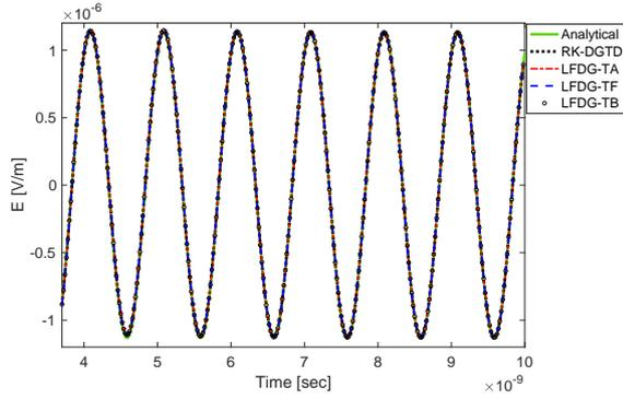
Fig. 2. Time-domain electric field at the observation point inside the conductive half-space.
