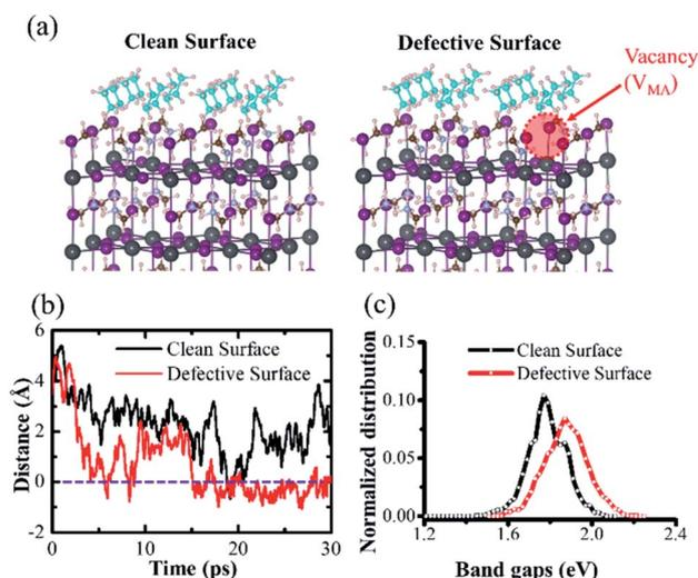
**Fig. 3** Model configurations (a) of both the clean perovskite surface and MAI-vacancy defective surface in AIMD simulations. (b) Distances between adsorbed  $\text{CH}_3\text{NH}_2$  (green color) and perovskite surfaces as a function of time (negative values represent the  $\text{CH}_3\text{NH}_2$  molecule penetrating into the perovskite surface). The energy distributions of optical band gaps (c) obtained from AIMD simulations.
