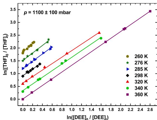
Fig. 1. Relative rate plots used to determine the rate coefficient ratio  $k_1 / k_4$  at different reaction temperatures using the OH + DEE (4) reaction as reference. The experimental data were fitted by Eq. (I), but the  $\ln([\text{THF}]_0 / [\text{THF}]_t)$  data are shifted for each temperature (at  $T < 360$  K) by + 0.3 unit for a better visualization.
