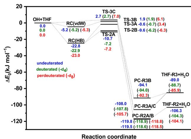
Fig. 4. Zero-point corrected CCSD(T)/cc-pV(T,Q)Z//MP2/aug-cc-pVDZ potential energies ( $\Delta E_0$ ) for the reactions OH + THF (1), OH + THF- $d_4$  (2) and OH + THF- $d_8$  (3); energies are relative to reactant energies.
