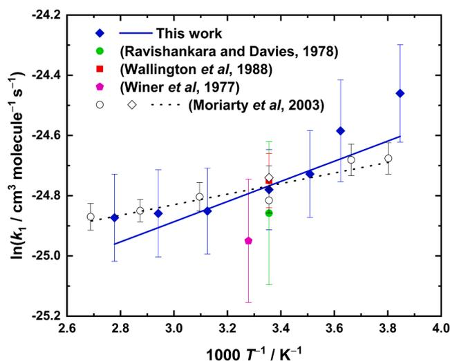
Fig. 3. Arrhenius plot for the temperature dependence of the rate coefficient for the reaction OH + THF (1) determined in current experiments and reported in the literature over the temperature range  $T = 260$ – $372$  K.
