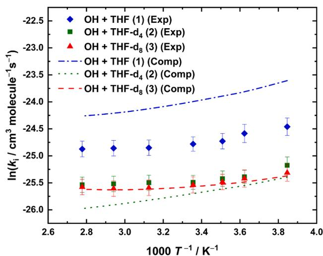
Fig. 5.  $\ln k_i$  vs.  $1/T$  ( $i = 1, 2, 3$ ) Arrhenius plots of experimental and computed rate coefficients for the reactions OH + THF (1), OH + THF-d<sub>4</sub> (2) and OH + THF-d<sub>8</sub> (3) in the temperature range of the experiments,  $T = 260\text{--}360$  K.
