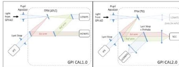
Fig. 3: Schematic view of our CAL 2.0 upgrades (right) compared to the CAL1.0 subsystem (left).
