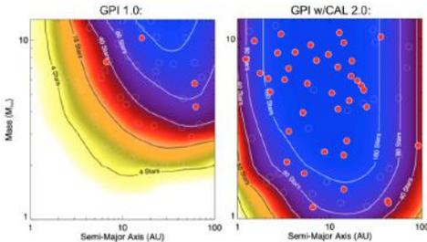
Fig. 1: Left panel, exoplanet sensitivity and detections for a 300-star survey using GPI1.0 and (right) for CAL2.0 as a science camera (credit: E. Nielsen). Detected planets in the sample are shown as red-filled circles, while undetected planets are shown as open white circles. The new CAL system is expected to increase the sensitivity to lower mass exoplanets at smaller separations.
