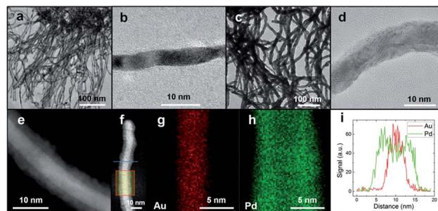
Fig. 2 Physical characterization of the vertically aligned NM nanowire forest. (a) TEM image of Au NWs. (b) HRTEM image of Au NWs. (c) TEM image of Au@Pd NWs. (d) HRTEM image of Au@Pd NWs. (e and f) HRSTEM image of Au@Pd NWs showing a clear core-shell nanostructure. (g and h) Electron energy loss spectroscopy (EELS) mapping of a single Au@Pd NW as displayed in (f). (i) Energy dispersive X-ray spectroscopy (EDX) line scan along the cross-section of a single Au@Pd NW as shown in (f).
