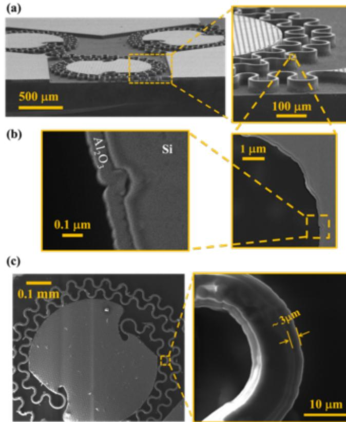
**Fig. 2** (a) SEM images of SAS structure after DRIE including zoom-in view. (b) SEM image of a representative defect of  $\sim 0.1 \mu\text{m}$  in size, found along one of the arms of a spiral (the conformal layer along the geometry is the  $\text{Al}_2\text{O}_3$  sidewall protection layer deposited in an earlier fabrication step). (c) SEM image of parylene-coated, SAS structure, including zoom-in of the arm showing the parylene thickness.
