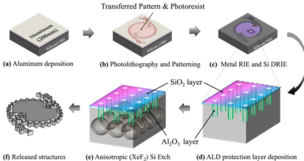
**Fig. 1** Fabrication process flow of SAS structure detailing (a) sputtering of Al, (b) photolithographic patterning of the structure, (c) the Al and the  $\text{SiO}_2$  RIE etching process, as well as the DRIE Si etch of the patterned structure, (d)  $\text{Al}_2\text{O}_3$  deposition on sidewalls, (e)  $\text{XeF}_2$  etch and (f) released silicon structure.
