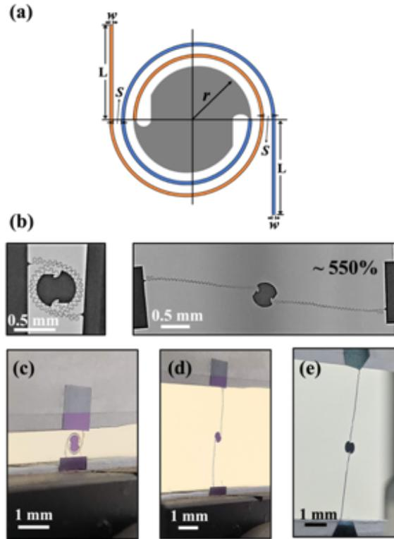
**Fig. 3** (a) Schematic diagram of straight-arm spiral. (b) Optical-microscope photographs of a un-stretched and stretched SAS structure up to  $\sim 550\%$  elongation, showing details of the serpentine-arms. (c) Un-stretched and (d) stretched SAS structure during tensile test, before fracture. (e) Fully stretched parylene-coated SAS compound structure. (Spiral arm's width is  $5 \mu\text{m}$  and  $N = 2$  for all cases).
