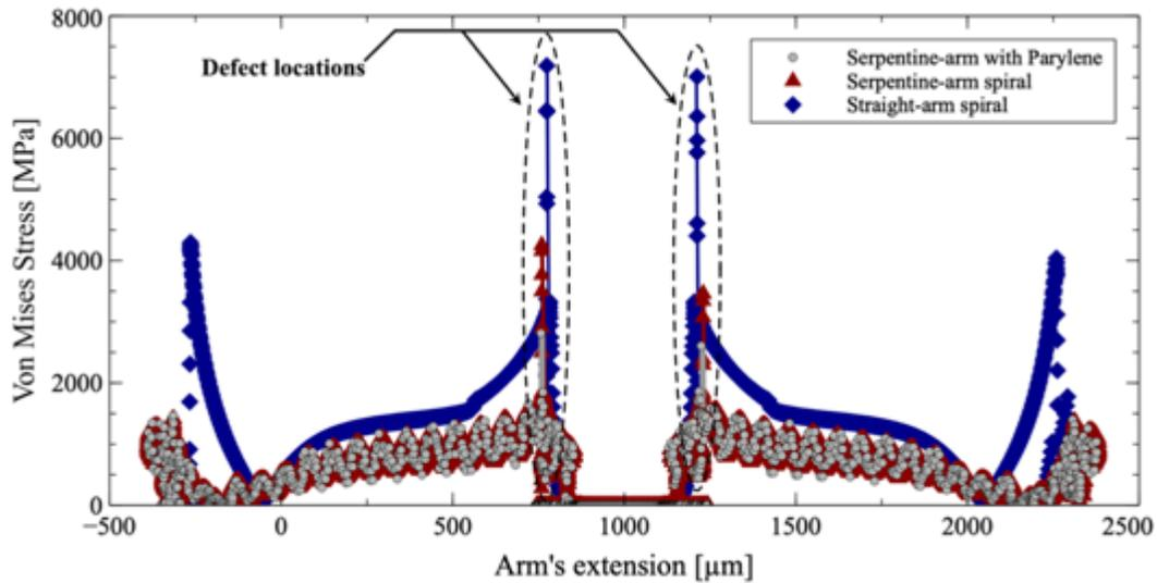
**Fig. 5** Comparison at 2 mm total displacement between the stress distribution along the arms of the straight-arm spiral, un-coated SAS and parylene-coated SAS structures. (Defects are located at the start of the arms with a size of 0.1  $\mu\text{m}$ ).
