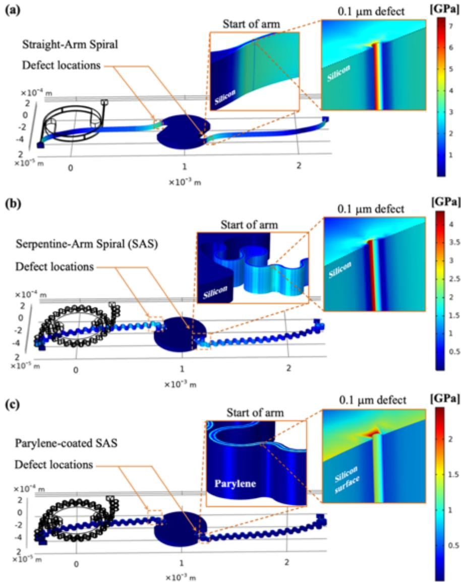
**Fig. 4** Von Mises stress distribution along different designs extended up to a 2 mm displacement, with  $0.1 \mu\text{m}$  defects located at the start of the arms. (a) Straight-arm spiral structure with zoom-in views at defect location. (b) SAS structure with zoom-in views at defect location. (c) SAS structure with parylene-coating and zoom-in views showing reduced stress concentration (Parylene was hidden from smaller inset to appreciate the stress at the silicon surface).
