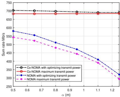
Fig. 4. The effect of increasing the interference at weak users on sum-rate.
