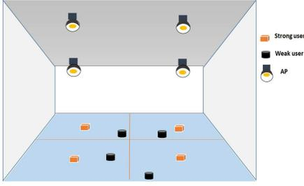
Fig. 1. An example of system model with 4 cells.
