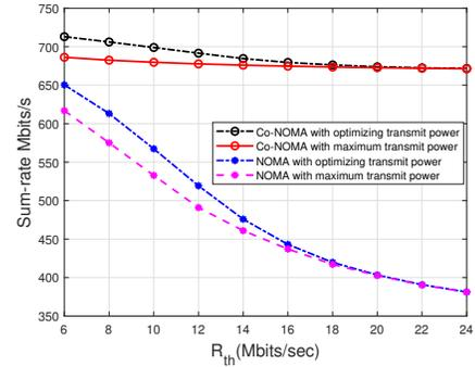
Fig. 2. The effect of  $R_{th}$  on sum-rate.
