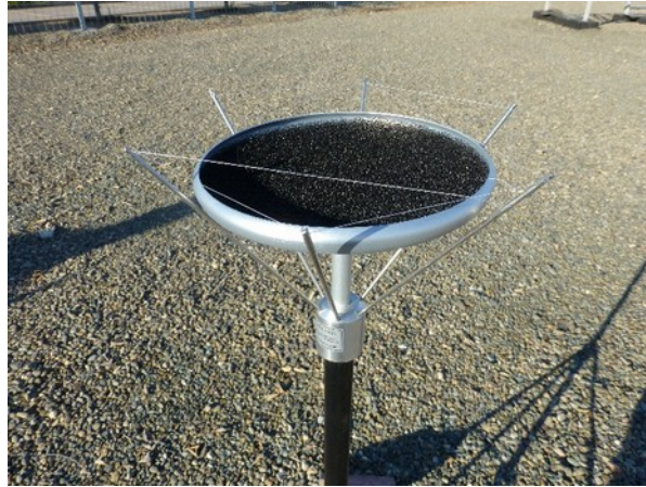
Fig. 1. Inverted Frisby aerosol deposition gauge, with polyester foam insert to prevent dust deposits being blown out once deposited in the dish. Also shown are spikes and fishing lines to discourage birds wanting to land on the sampler.
