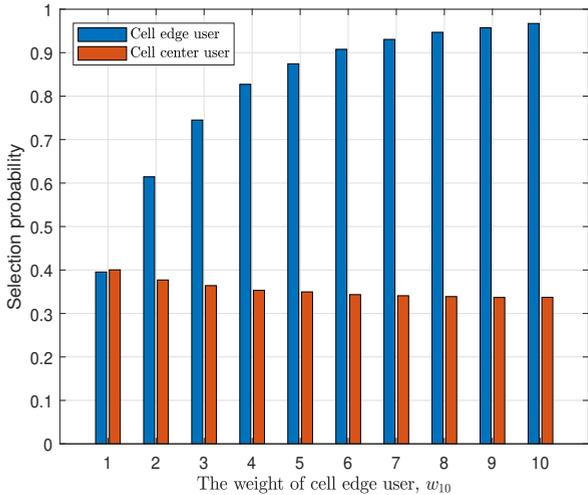
(a) Selection probability versus the weight of user at cell edge.
