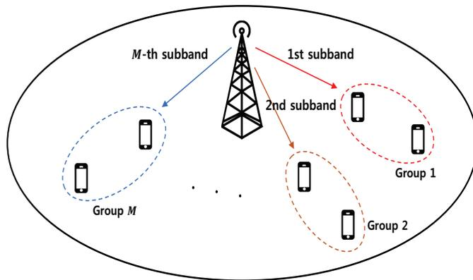
FIGURE 1: Multiple access systems combining NOMA with conventional FDMA.
