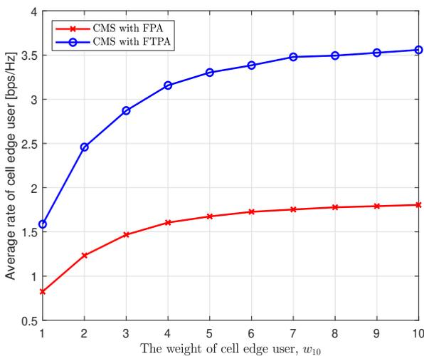
(b) Average rate versus the weight of user at cell edge with FPA and FTPA.
