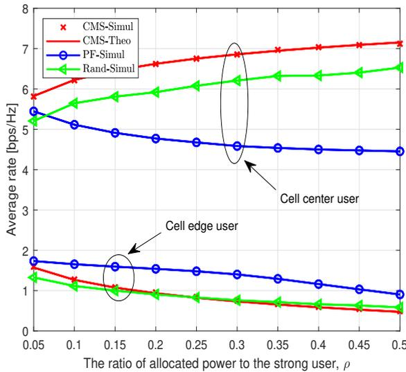
FIGURE 4: Performance of the average rate in terms of the ratio of allocated power to the strong user,  $\rho$ .
