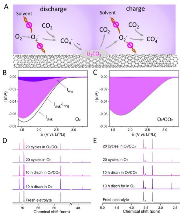
**Figure 3.** Schematic and confirmation of CO<sub>2</sub> endowed cathode and electrolyte stabilization in Li-O<sub>2</sub>/CO<sub>2</sub> batteries. (A) The proposed reaction route of capturing O<sub>2</sub> by CO<sub>2</sub>. (B, C) The RRDE experiments in O<sub>2</sub> and O<sub>2</sub>/CO<sub>2</sub> with 0.1 M LiCF<sub>3</sub>SO<sub>3</sub>/TEGDME electrolyte. (D, E) <sup>13</sup>C and <sup>1</sup>H NMR spectra of the cycled electrolytes dissolved in D<sub>2</sub>O.
