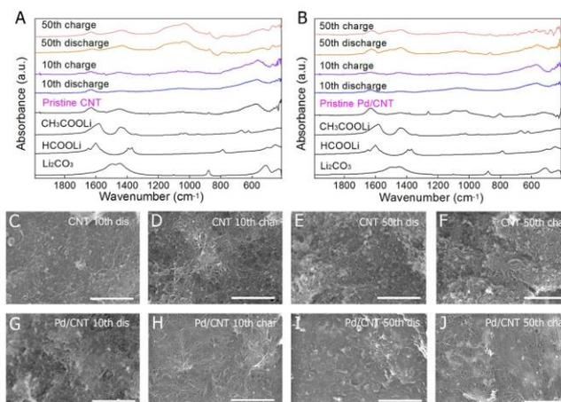
**Figure 4.** FTIR spectra and SEM pictures of cycled CNT and Pd/CNT cathodes at the end of discharge and charge states. (A, B) FTIR spectra of CNT and Pd/CNT cathodes. (C-F) SEM pictures of CNT. (G-I) SEM pictures of Pd/CNT. The batteries were cycled with a cutoff capacity of 1000 mAh g<sup>-1</sup> at 500 mA g<sup>-1</sup>. Scale bar: 2 μm.
