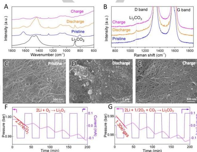
**Figure 1.** The rechargeability of Li-O<sub>2</sub>/CO<sub>2</sub> battery. (A) FTIR spectra and (B) Raman spectra of the pristine, discharged and charged cathodes. (C-E) The corresponding SEM pictures of the cathodes. (F) The pressure change during cycling of Li-O<sub>2</sub> battery. (G) The pressure change during cycling Li-O<sub>2</sub>/CO<sub>2</sub> battery. Current density is 0.1 mA (88.5 μA cm<sup>-2</sup>) for F and G.
