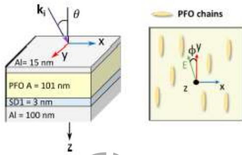
Representation of a TE-polarized wave incident on a microcavity containing an oriented layer of PFO, details on the geometry can be found in the main text.
