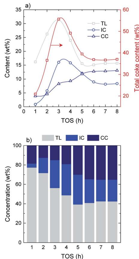
Fig. 3 Evolution with TOS of the (a) amount of total coke and the different coke species and (b) concentration of the different deactivating species in coke.
