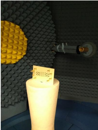
Fig. 2. Measurements of the antenna array inside the chamber.
