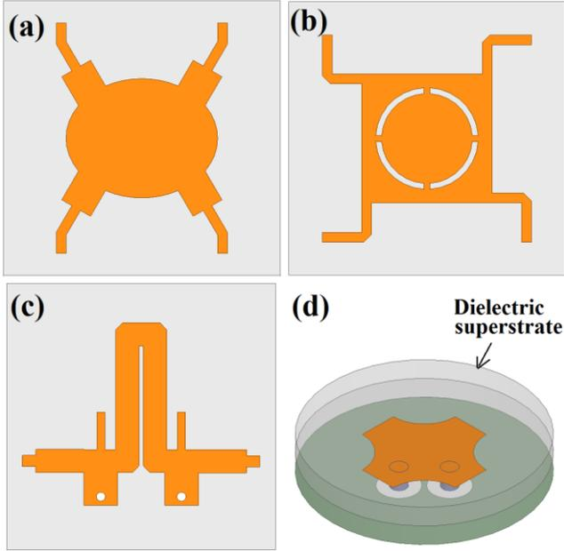
Fig. 1. (a) the quadrature 3-dB directional coupler; (b) the crossover; (c) the phase shifter; (d) the radiating patch element.
