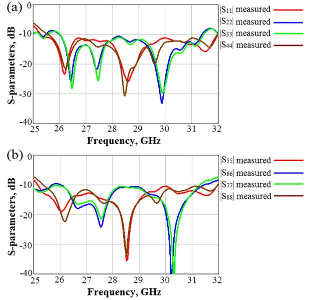
Fig. 3. The measured reflection coefficients: (a) for ports 1-4, (b) for ports 5-8.
