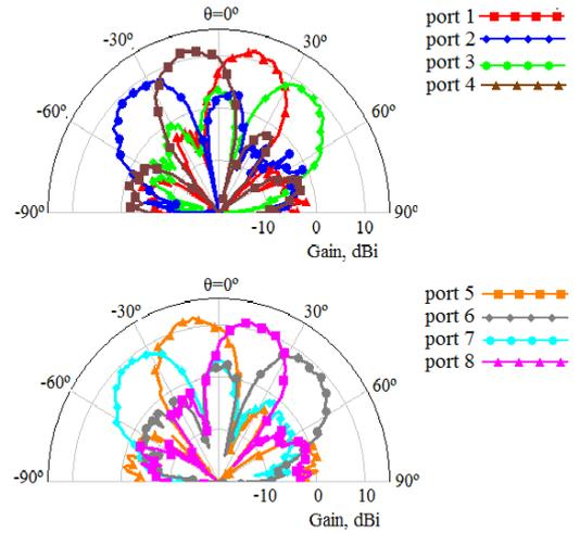
Fig. 4. Measured radiation patterns of the antenna at 28 GHz.
