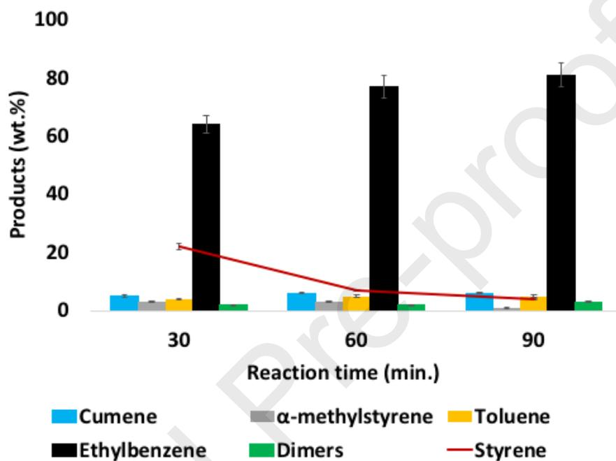
**Figure 4** Exposure time effect on the transformation of PS into EB (Conditions: reaction temperature 250 °C, catalyst weight: 0.20 g, PS weight: 2.0 g, and under air).
