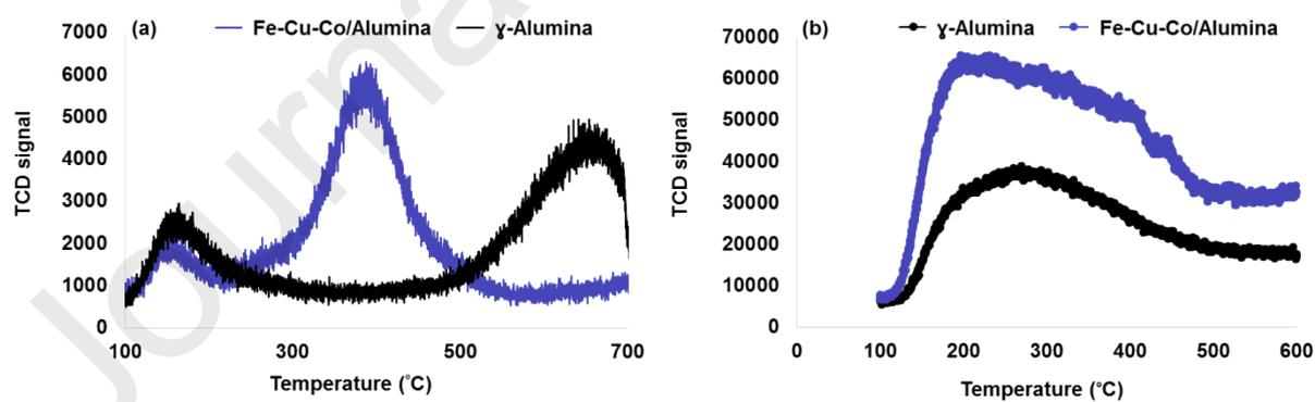
**Figure 1** Temperature program desorption of Fe-Cu-Co/Alumina and Alumina (a) CO<sub>2</sub> TPD and (b) NH<sub>3</sub> TPD.
