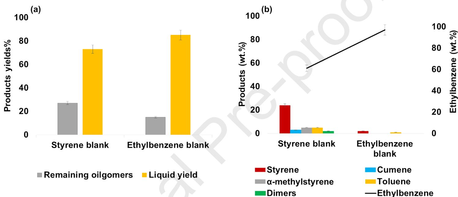
**Figure 3** Control experiments of styrene and ethylbenzene reactivity in the presence of Fe-Cu-Co/Alumina (a) product yields and (b) Products selectivity in wt.% (Conditions: reaction temperature 250 °C, catalyst loading: 0.20 g, exposure time: 90 min., and under air).
