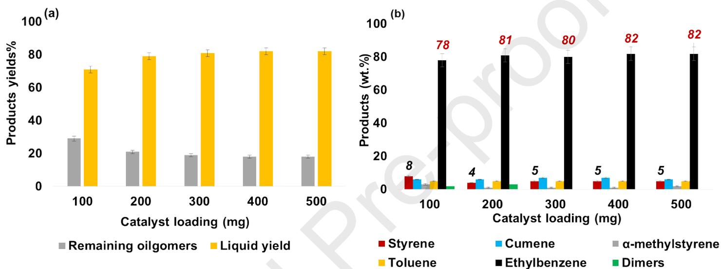
**Figure 5** Fe-Co-Cu/Alumina loading effect on the products selectivity (Conditions: reaction temperature 250 °C, exposure time: 90 min., PS loading: 2.0 g, and under air).
