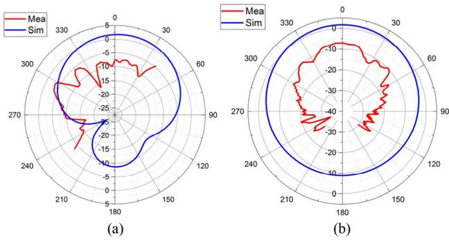
Fig. 5. Measurement results and simulation results of radiation patterns (a) E-plane (b) H-plane
