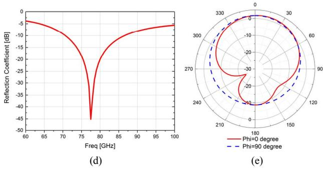
Fig. 1. (a) HFSS simulation model of CPW-fed monopole on-chip antenna (b) Microscope view of the chip (c) standard 0.18 $\mu$ m stack-up (d) simulation result of the reflection coefficient (e) simulation result of radiation pattern
