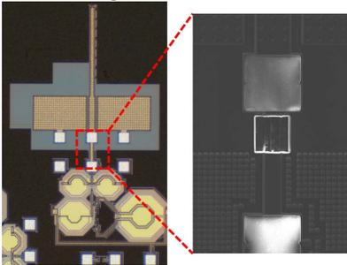
Fig. 2. Transmission line cut by FIB
