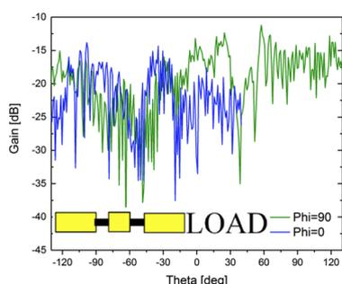
Fig. 8. Probe tip radiation (50 Ω loaded)
