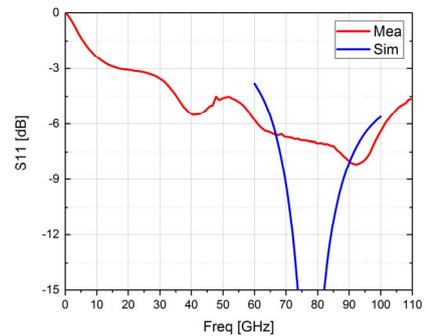
Fig. 4. Measurement result and simulation result of antenna return loss
