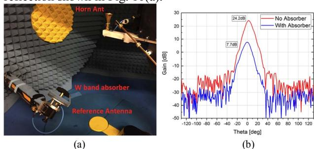
Fig. 9. (a) Absorber performance measurement setup (b) Absorber performance measurement results
