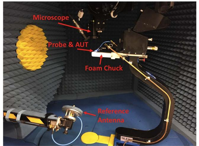
Fig. 3.  $\mu$ -Lab mm-wave anechoic chamber
