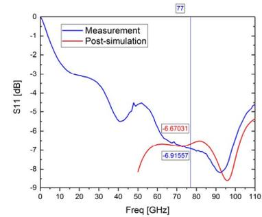
Fig. 7. Reflection coefficients of measurement and post-simulation
