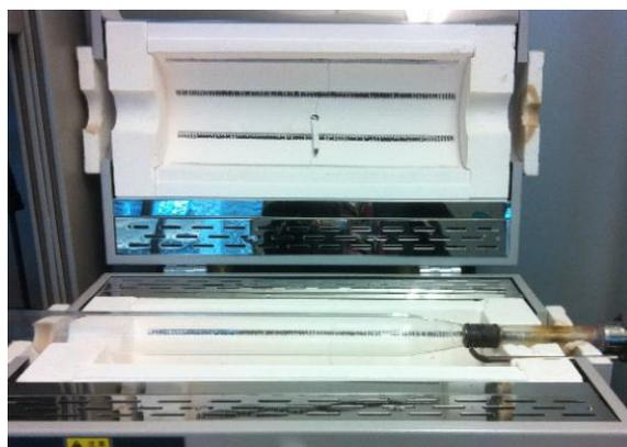
Fig. 1 Temperature controlled DBD reactor.
