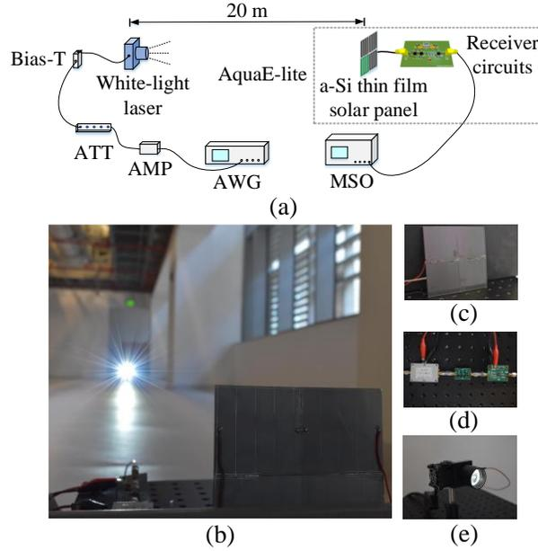
Fig. 1. (a) Experimental setup of the white-light laser and a-Si thin-film solar panel-based VLC system, (b) experimental scene, (c) a-Si thin-film solar panel, (d) receiver circuits, and (e) white-light laser.
