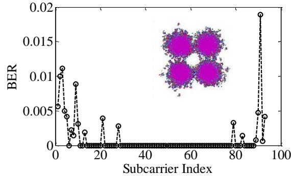
Fig. 9. BERs of the received OFDM signals for different subcarriers over 2.4-m outdoor pool water. Inset: the corresponding constellation map.
