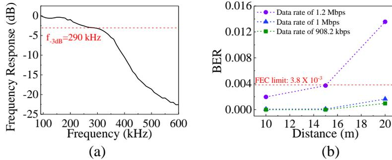
Fig. 5. (a) Frequency response of the whole system measured at a transmission distance of 20 m, and (b) BERs of 908.2-kb/s, 1-Mb/s, and 1.2-Mb/s 4-QAM OFDM signals at transmission distances of 10, 15, and 20 m.
