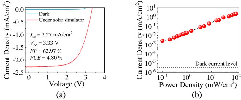
Fig. 2. (a)  $J$ - $V$  curve of an a-Si thin-film solar cell in the dark and under an illumination intensity of  $100 \text{ mW/cm}^2$  using the AM 1.5 G solar simulator, and (b) current densities of the a-Si thin-film solar cell under different power densities.
