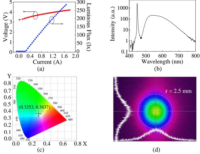
Fig. 3. (a)  $L$ - $I$ - $V$  characteristics of the white-light laser, (b) optical spectrum of the white-light laser under a drive current of 570 mA, (c) CIE 1931 diagram with chromaticity coordinates ( $x$ ,  $y$ ) of the white-light laser, and (d) beam shape and power distribution of the white-light laser.
