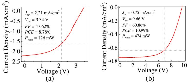
Fig. 7. Under an illumination intensity of  $40 \text{ mW/cm}^2$ , (a)  $J$ - $V$  curve of one single a-Si thin-film solar cell and (b)  $J$ - $V$  curve of three a-Si thin-film solar cells connected in series.
