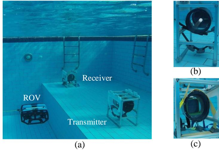
Fig. 8. (a) Experimental scene, (b) transmitter: white-light laser, and (c) receiver: AquaE-lite.
