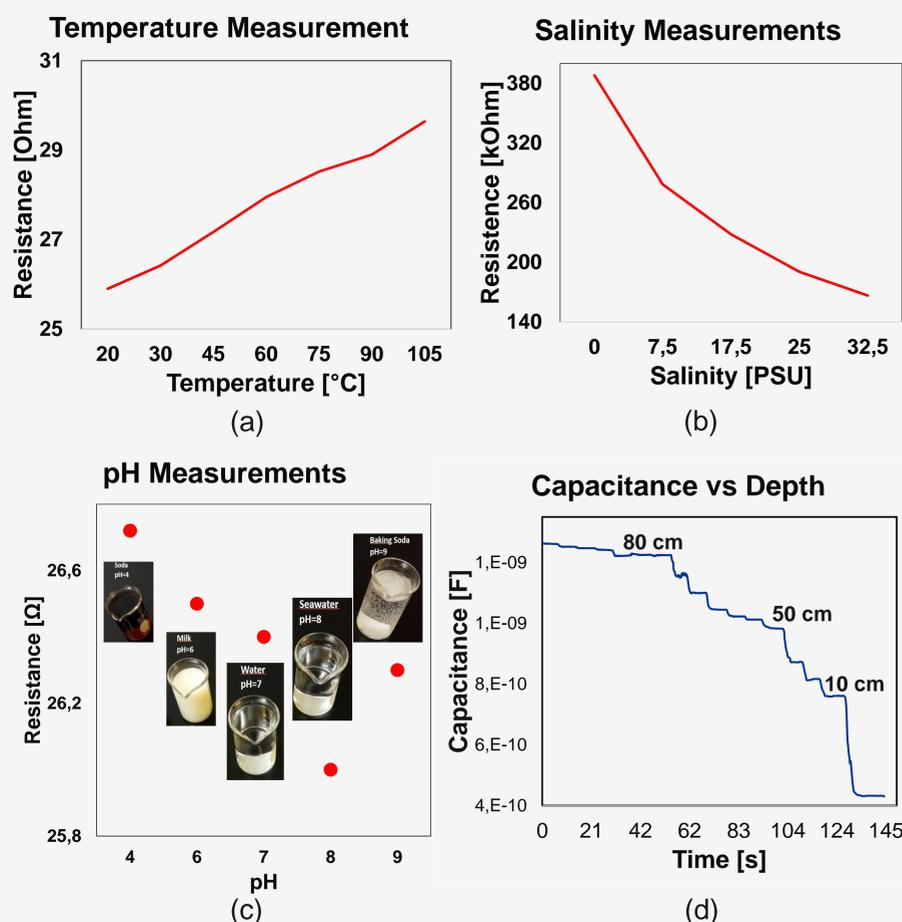
Laboratory tests: (a) Resistance vs Temperature for Gold; (b) Copper pattern resistance vs Water salinity; (c) Resistance of Copper pattern covered with Graphene vs pH; (d) Sensor capacitance vs Sensor Depth.
