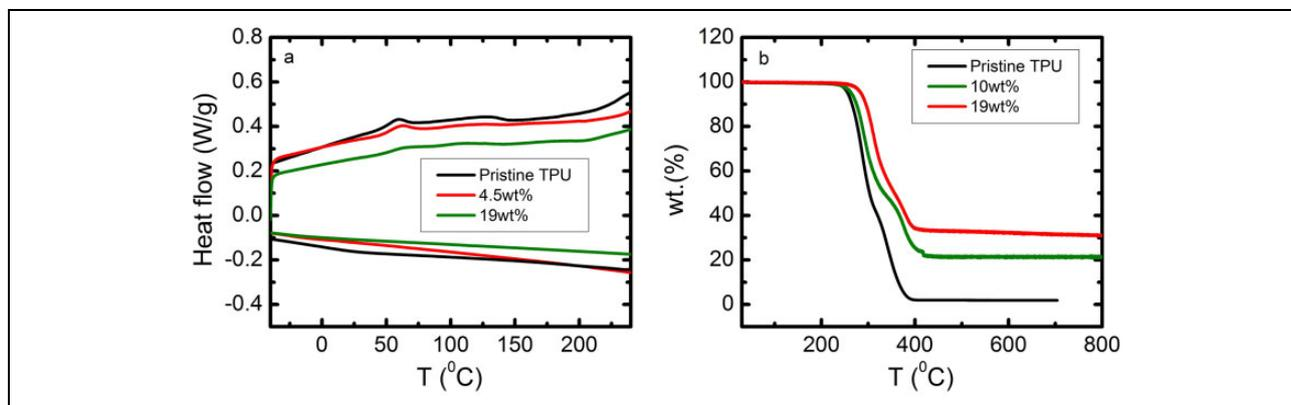
**Figure 5.** (a) DSC measurements of polymer and composites show reduction in polymer crystallization in the composite with increasing nanotube concentration. (b) TGA of nanotubes, polymer and composites under atmospheric air. DSC: differential scanning calorimetry; TGA: thermogravimetric analysis.
