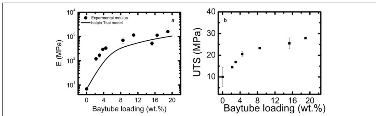
**Figure 3.** Mechanical characteristics of composites. (a) The values of  $E$  (black solid circles) of the composites increase by >20,000% with loading of 19 wt% of nanotubes. The enhancement in  $E$  is well-predicted by the Halpin–Tsai model (block solid line). (b) The UTS of the composites (black solid square) also increases with the loading of nanotubes. The error bars are obtained from measurements on multiple samples.  $E$ : tensile modulus; UTS: ultimate tensile strength.
