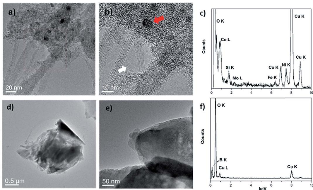
**Fig. 1** (a and b) TEM micrographs of the as-received SWCNT-1, where the white arrow points to a single nanotube, while the red arrow marks a catalyst particle; (c) EDS of the sample in (a); (d and e) TEM micrographs of a typical aggregate found in the fusion residues of the SWCNT-1 mixture; (f) EDS of (d). Please note that the Si and Cu peaks in the spectra of (c) and (f) originate from the sample grid.
