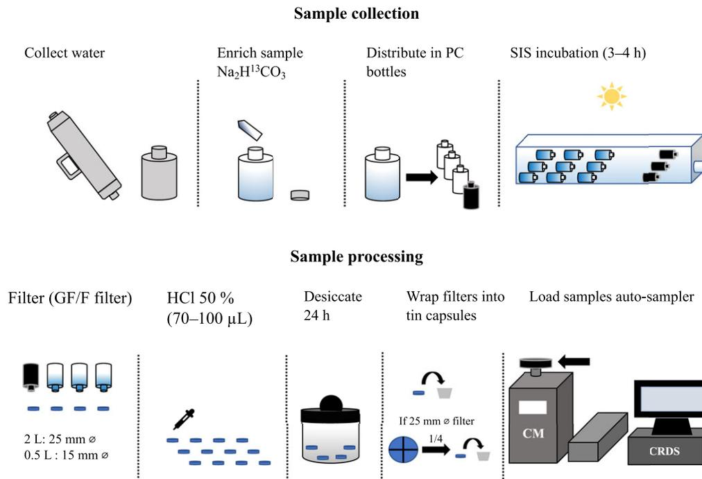
**Fig. 2.** Schematic representation summarizing the different steps to collect and process samples for primary production measurements using the <sup>13</sup>C-CRDS-PP method.
