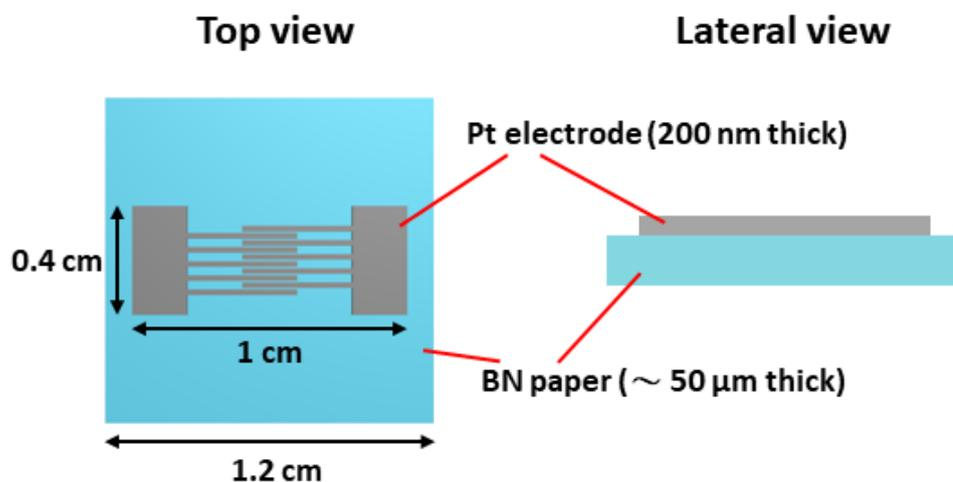
**Fig. S1** Top view and lateral view illustration of BN paper PD structure
