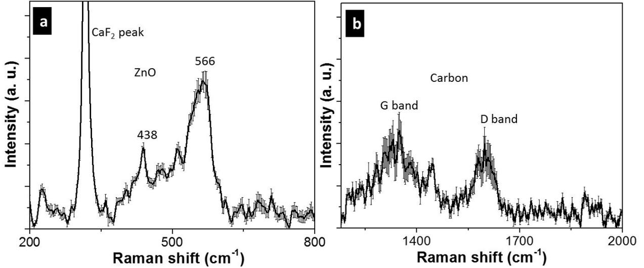
**Figure S2.** Raman spectrum of C-doped ZnO QDs. (a) Raman spectra originating from ZnO QDs and (b) spectra showing presence of G and D band of carbon.
