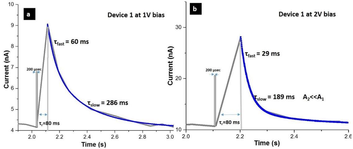
**Figure S4.** The calculation of the rise time and the decay time of Device 1 at the applied bias of (a) 1 V and (b) 2 V.
