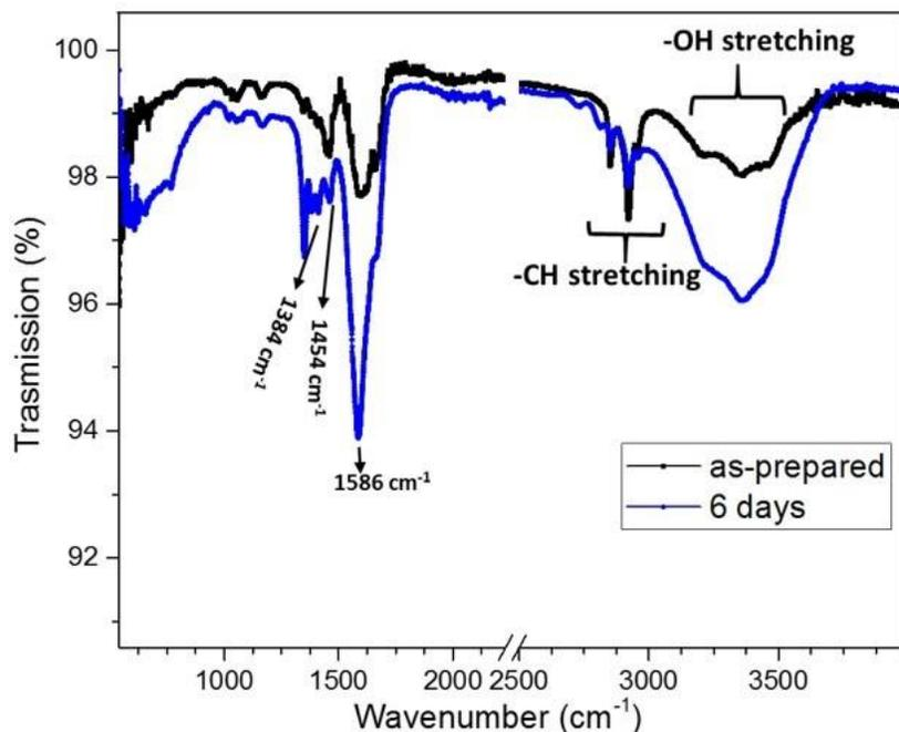
**Figure S1.** Fourier transform infrared transmission signal of as-prepared ZnO QDs and QDs aged in ethanol.
