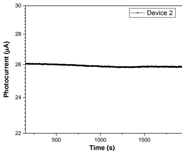
**Figure S7.** Photocurrent of the device 2 under 224 nm continuous illumination.
