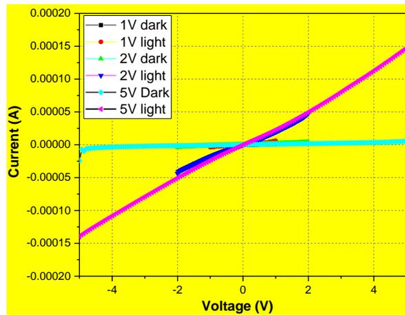
**Figure S6.** The I-V curve of Device 1 with and without CW 224 nm illumination was measured by Kiethley 2400 sourcemeter. 1000 W Xenon (Newport 66923) white light source was coupled with monochromator to produce 224 nm illumination, as our pulsed laser cannot be used for I-V measurements.
