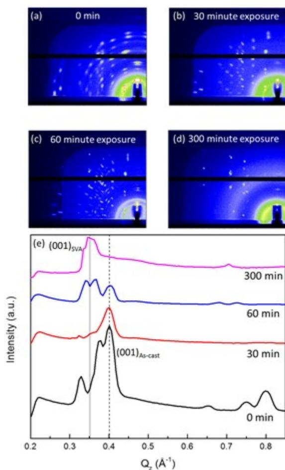
**Figure 4.** In-situ GIXD patterns of (a) spin-coated BT film before exposure to chlorobenzene vapors. (b) Film after 30 minutes, (c) 60 minutes, and (d) 300 minutes of SVA. (e) Out-of-plane intensity plots with lines to guide the eye along the major diffraction peak of the as cast (dashed) and static solvent annealed films
