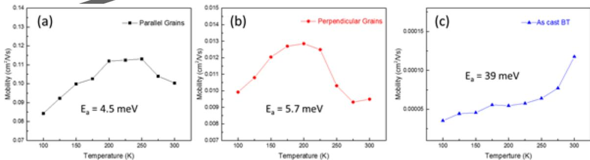
**Figure 8.** Temperature-dependent saturation mobility ( $V_D = -60$  V) measured in 50  $\mu\text{m}$  channel of (a) solvent-annealed parallel grains, (b) perpendicular grains, and (c) as cast film. The activation energies ( $E_a$ ) extracted in the trap dominated regimes are also given.
