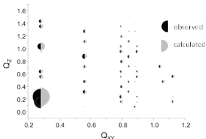
**Figure 2.** The measured and calculated diffraction intensities (best-fit) for the spin coated BT film.
