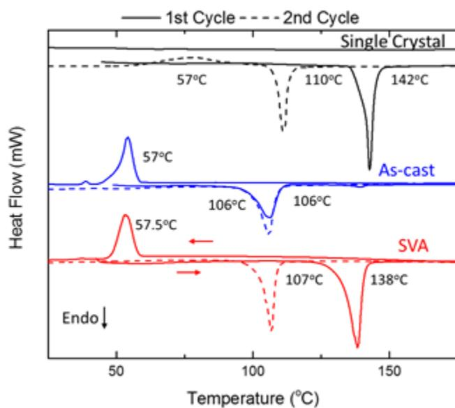
**Figure 5.** Heating (solid), cooling (solid), and 2nd heating (dashed) thermograms of BT in the single crystal (black), drop casted (blue), and solvent vapor annealed (red); heating rate, 10 °C/min.
