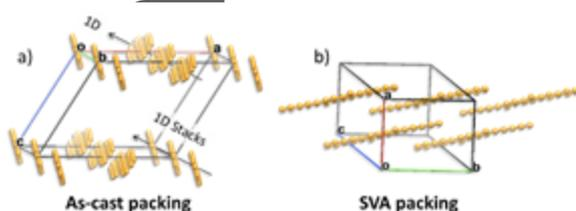
**Figure 3.** Crystal structure and molecular packing of (a) as-cast BT polymorph. The 1D pi-stacks crystallize along the b-axis (010). (b) The solvent vapor annealed BT molecular packing is identical to the bulk crystal structure (2D brick layer motif). Note: the silylethynyl solubilizing groups have been removed for clarity.
