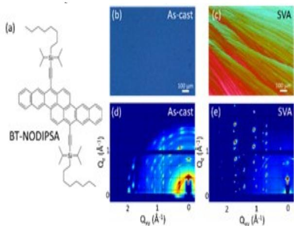
**Figure 1.** a) Chemical structure of BT, (b) optical image of a spin-coated film of BT, and (c) polarized optical image of BT film after solvent vapor annealing. (d) 2D-GIXD patterns of the as-cast BT and (e) SVA films.
