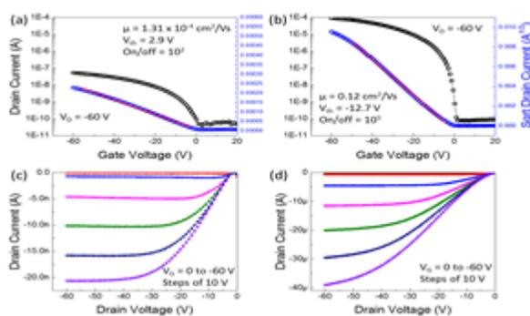
**Figure 6.** (a) Transfer characteristics in the saturated region of the as cast BT film and (b) SVA film. (c) Output characteristics of the as cast BT and (d) SVA film.
