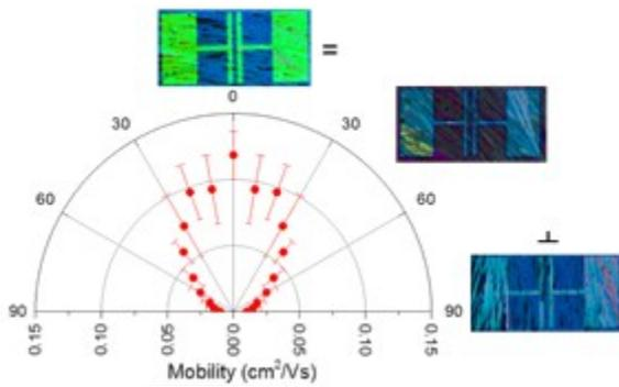
**Figure 7.** Polar plot of the hole mobility versus grain orientation angle of solvent vapor annealed BT film. The mobility data is reported from 0° to 90° and reflected to show the expected behavior over 180°. Devices with grains oriented at 0° are denoted as parallel, and grains oriented 90° to the channel are denoted as perpendicular
