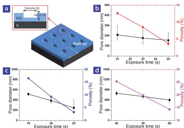
Fig. 1 (a) Schematic of the NP SiO<sub>2</sub>/Si substrate. Pore diameter and porosity vs. exposure time at different pitches of (b) 500 nm, (c) 1000 nm, and (d) 1500 nm. The pitch was controlled by the interference angle between the two beams, and the pore diameter was determined by the exposure time and development time. All the samples were used as a gate dielectric layer for the following bottom-contact G-FETs.
