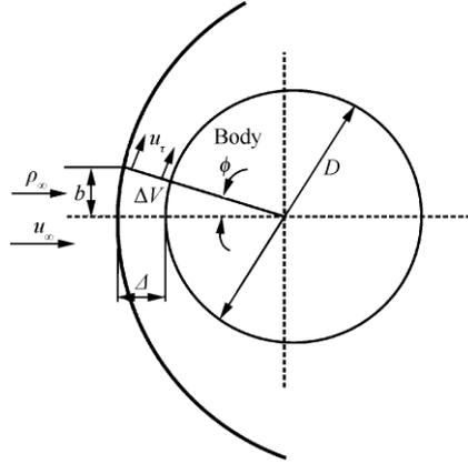
Fig. 1 Schematic of control volume and associated notations.
