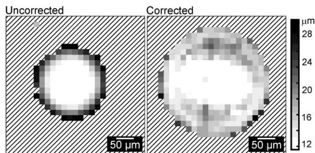
Figure 1: Axial resolution as a function of position in the x,y plane for uncorrected (left) and corrected (right) endoscopic probes (probe length: 1.86 mm; probe diameter: 0.5 mm). The grey scale indicates axial resolution values in microns measured with the technique described in [2].
