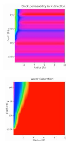
Radial applications involve field variables such as mud density, overbalance pressure and pump rate. The grid permits the presence of high permeability channels (discrete fractures). Optimizing particle size distributions for a specific case, invasion radius could be reduced up to 70%. Furthermore, production constraints effect on permeability return can be assessed with final skin/permeability profiles along the well.
