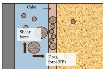
Cake thickness controls the filtration rate (inner boundary condition) and it is determined by balancing forces (axial and radial forces) and petrophysical characterization. Cake growth is treated explicitly and is updated at every step.
