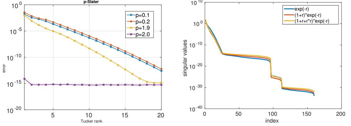
Figure 3.5: Convergence in the Frobenius error (3.26) w.r.t. the Tucker rank for the function (3.27) with  $p = 0.1, 0.2, 1.9, 2.0$  (left); Decay of singular values of the weighted Slater function (right).
