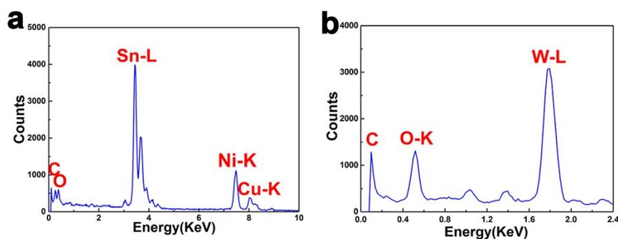
**Figure S1.** EDX spectra: (a) 97Sn3Cu nanosolders. (b) WO<sub>3</sub> nanowires.
