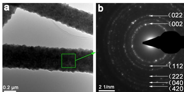
**Figure S2.** TEM structural analysis of  $\text{WO}_3$  nanowires. (a) A representative TEM image of  $\text{WO}_3$  nanowires. (b) A typical SAED pattern recorded from the area marked by the green square in (a).
