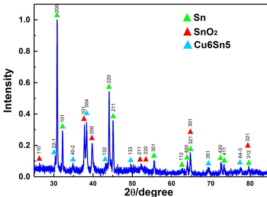
**Figure S3.** XRD pattern of the prepared 97Sn3Cu nanowires released from the PC template.
