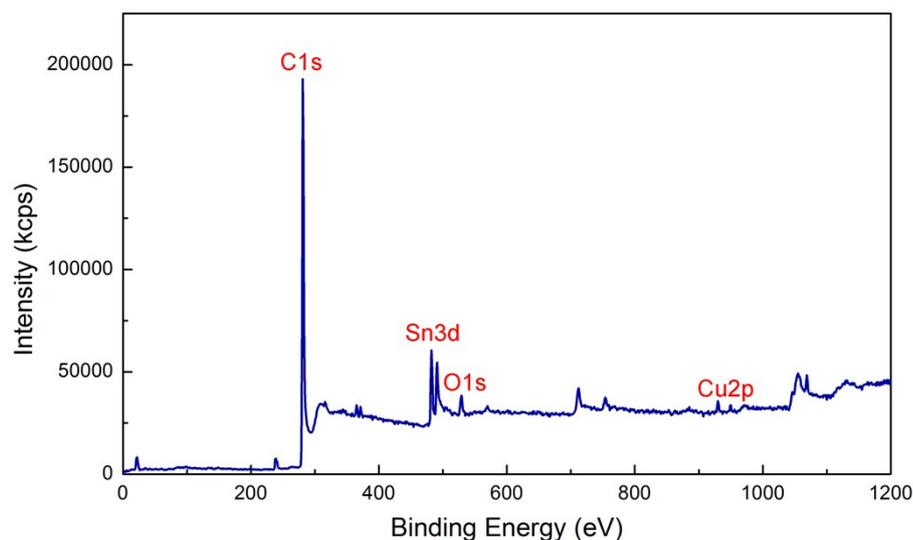
**Figure S5.** XPS wide spectrum after Ar ion sputtering 97Sn3Cu nanosolder for 110s
