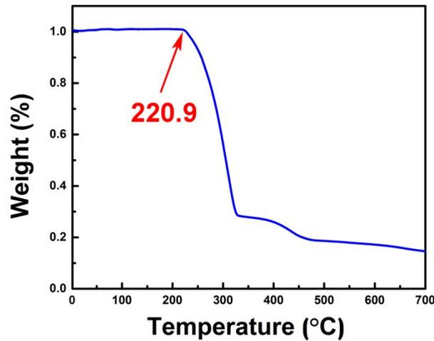
**Figure S4.** Thermogravimetric analysis curve of 97Sn3Cu nanosolder.
