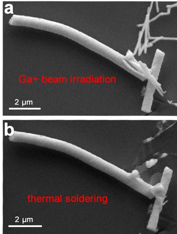
**Figure S7.** Thermal soldering two individual  $\text{WO}_3$  nanowires using  $97\text{Sn}3\text{Cu}$  nanowire solders. (a)  $\text{Ga}^+$  beam irradiation of the bundle of  $97\text{Sn}3\text{Cu}$  nanowires placed in the soldering point. (b) Thermal soldering the  $\text{WO}_3$  nanowires together after preheating at  $180\text{ }^\circ\text{C}$  for 2 min and followed reflow heating at  $250\text{ }^\circ\text{C}$  for 3 min.
