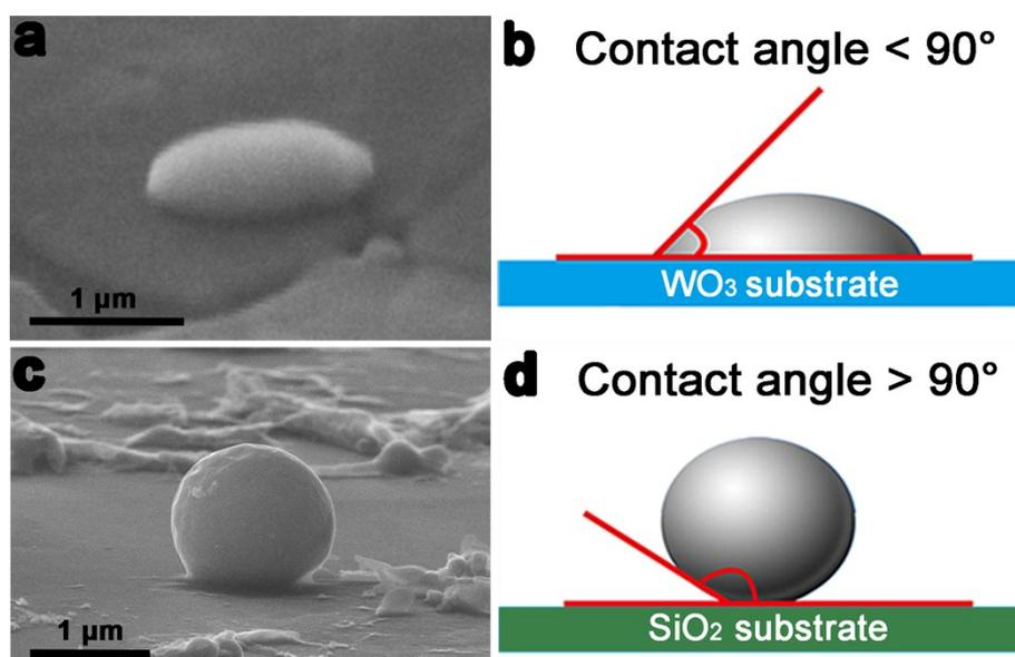
**Figure S6.** (a) The lateral profile SEM images of melted 97Sn3Cu nanosolder sphere on WO<sub>3</sub> substrate. (b) The schematic diagram corresponding to (a). (c) The lateral profile SEM images of melted 97Sn3Cu nanosolder sphere on SiO<sub>2</sub> substrates. (d) The schematic diagram corresponding to (c).
