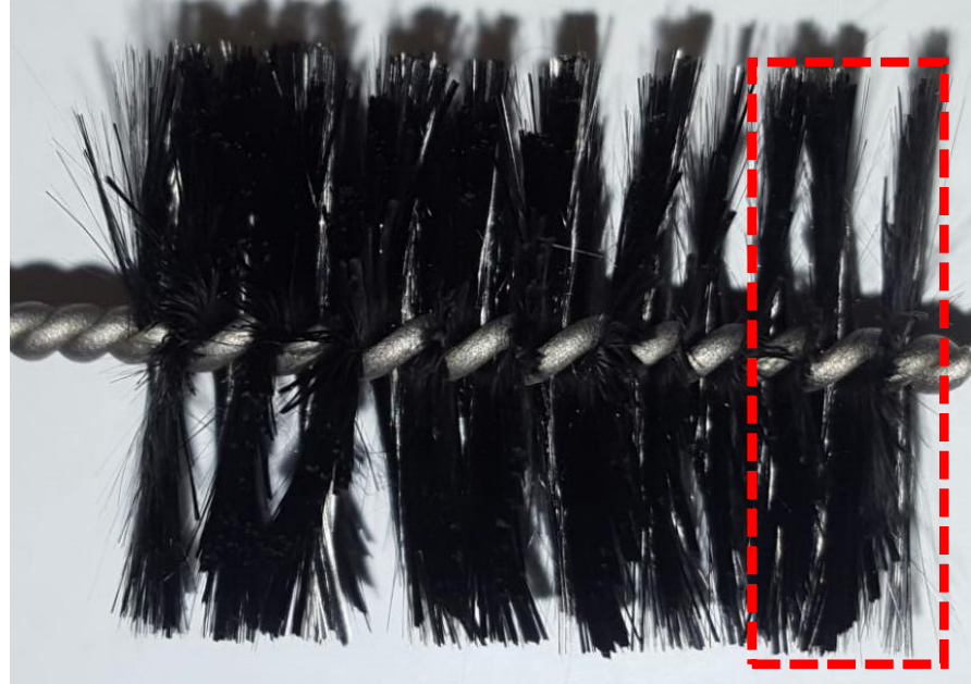
Supplementary Figure S1. Photo of the brush anode used in this study. The dashed rectangle represents the section of the anode that was sampled for microbial analysis.
