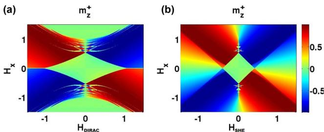
FIG. 2. Calculated switching phase diagram with an applied in-plane field along  $\mathbf{x}$  for a current-induced (a) Dirac torque and (b) spin Hall torque (retrieve results from Ref. [8])
