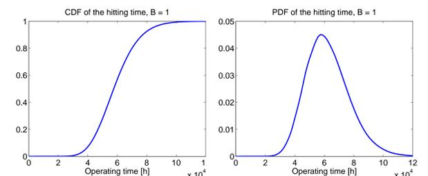
**Figure 6:** Left panel: CDF of the hitting time for  $B = 1$ . Right panel: PDF of the hitting time to the critical level.
