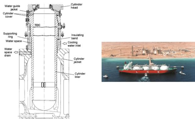
**Figure 1:** Left: Cross-section of the cylinder liner of a SULZER RTA 58 engine. Right: Data refer to cylinder liners, equipping natural gas transport ships like the one shown here.
