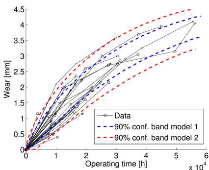
**Figure 2:** Data and 90% confidence bands for models 1 and 2. The confidence band for the model 2 is essentially the same as the one obtained by Giorgio et al. in [2] using a stochastic differential equation driven by gamma noise.
