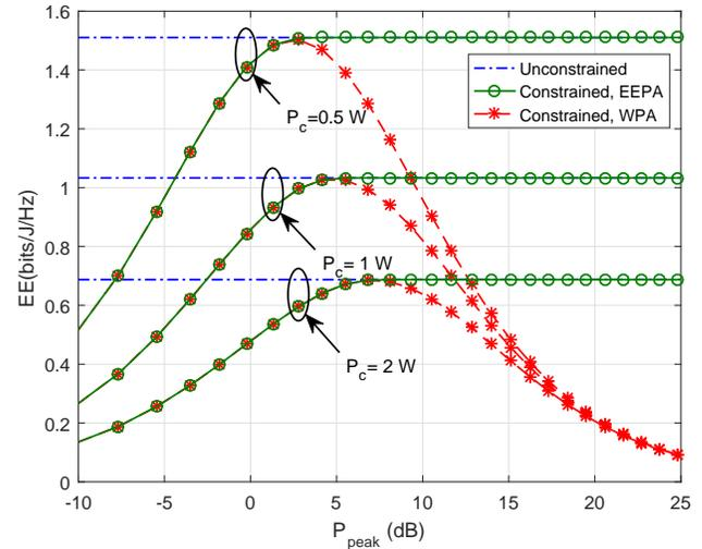
Figure 6: Constrained EE as a function of  $P_{peak}$  for different values of  $P_c$  with  $N = 4$  with no minimal rate constraint.
