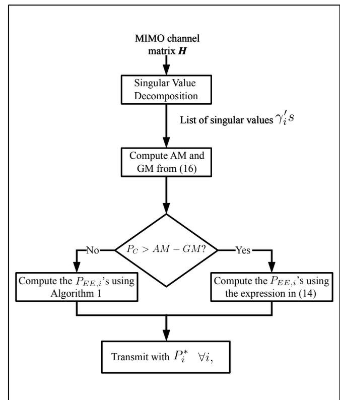
Figure 1: Illustration of the energy-efficient power allocation for the unconstrained MIMO-SVD systems.
