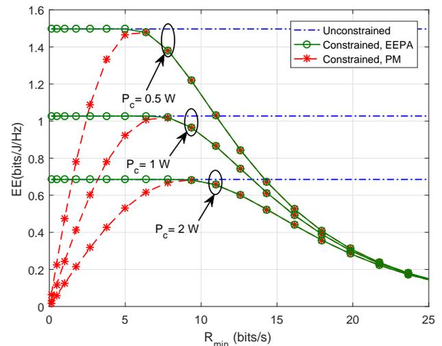
Figure 7: Constrained EE as a function of  $R_{min}$  for different values of  $P_c$  with  $N = 4$  with no power budget constraint.
