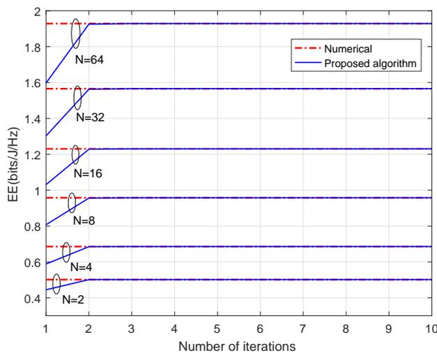
Figure 3: Unconstrained EE as a function of the number of iterations of Algorithm 1 with different values of  $N$  and  $P_c = 1$  W.
