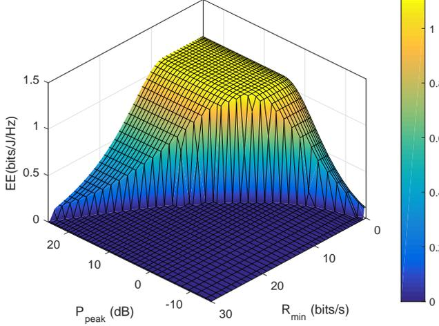
Figure 8: Illustration of the constrained EE as a function of  $P_{peak}$  and  $R_{min}$  for different values of  $P_c = 1$  W with  $N = 4$ .
