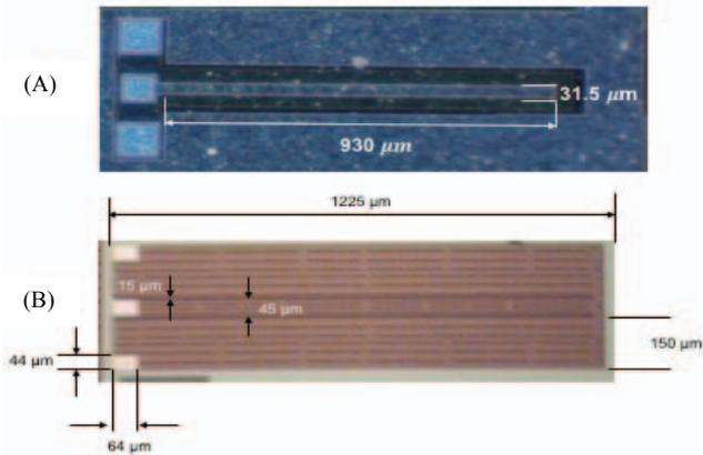
Fig. 1. (A) the microstrip line (TRL) and (B) Coplanar waveguide (CPW).
