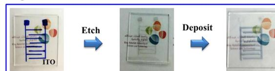
Transparent, electrochromic on-chip microsupercapacitors
