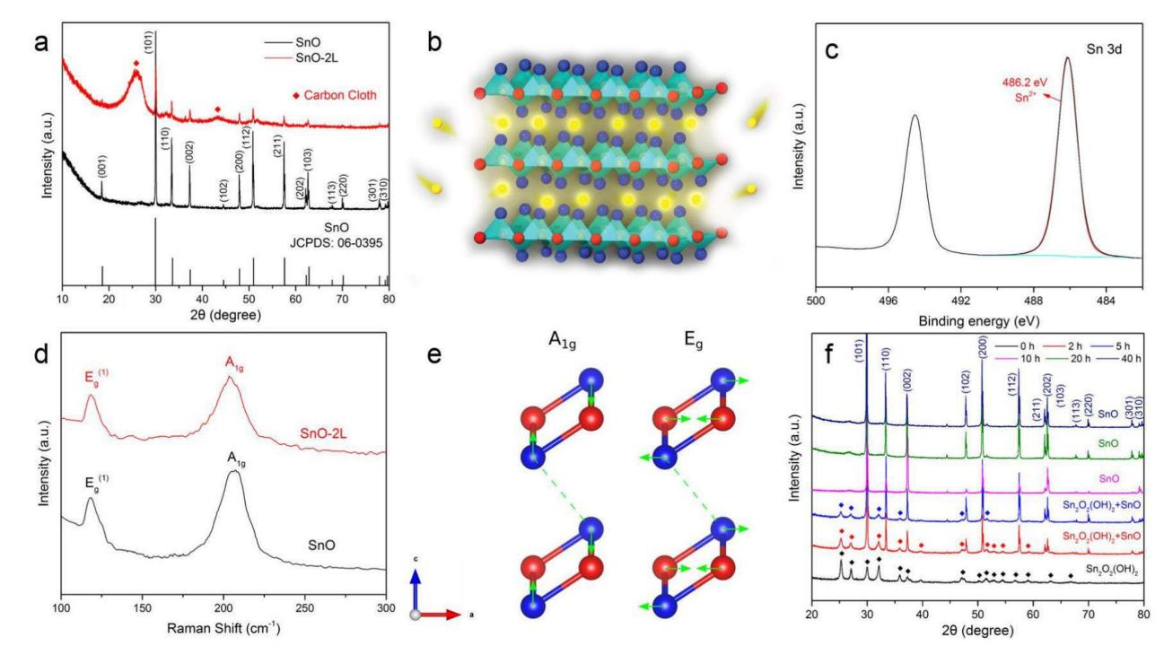
\* XRD, Raman and XPS tests have been utilized to demonstrate the successful synthesis of pure SnO powder and SnO@CC with different layers.
