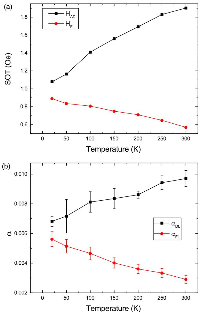
FIG. 4. (a) Temperature dependence of the effective field induced by dampinglike torque and fieldlike torque. (b) Temperature dependence of the electrical efficiency defined as  $\alpha_{\text{DL,FL}} = \frac{H_{\text{DL,FL}}}{J_c} \frac{M_s t_{\text{FM}}}{\hbar/2e}$ .
