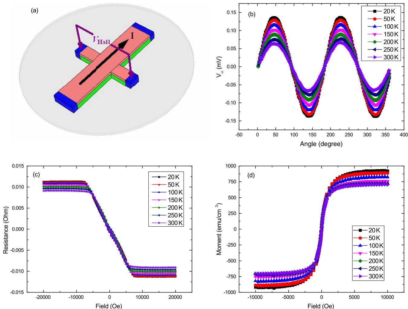
FIG. 1. (a) Schematic of the measurement geometry. (b) The first harmonic voltage  $V_\omega$  as a function of the azimuthal angle  $\varphi$  (PHE) at different temperatures. (c) Anomalous Hall resistance as a function of the external field measured at various temperatures. (d) The magnetization curves of  $\text{NiFe}$  (1.5) as a function of temperature.
