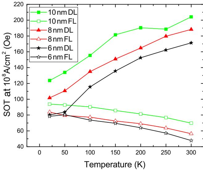
FIG. 5. Thickness dependence of the effective field induced by dampinglike torque and fieldlike torque. The filled and unfilled symbols indicate dampinglike and fieldlike torque, respectively. All current densities are converted to  $10^8$  A/cm<sup>2</sup>.
