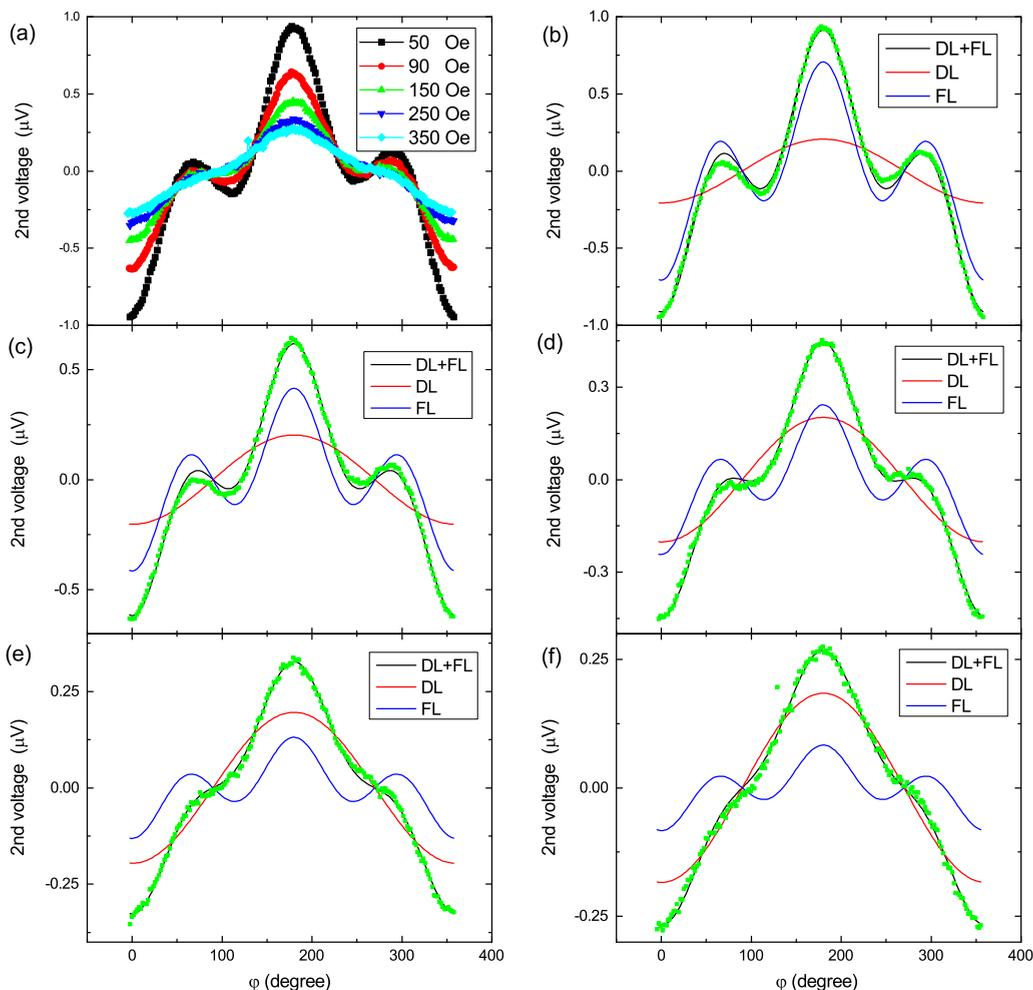
FIG. 2. (a) Second harmonic voltage  $V_{2\omega}$ , as a function of the azimuthal angle  $\phi$ , measured at 300 K. (b)–(f) Fitting by Eq. (2) from 50 to 350 Oe. The red line is the  $\cos \phi$  term, i.e., the dampinglike torque. The blue line is the  $2\cos^3 \phi - \cos \phi$  term, i.e., the fieldlike torque.
