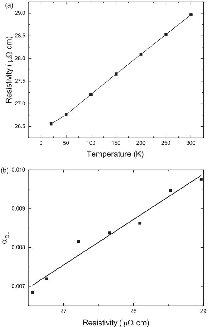
FIG. 6. (a) Resistivity of CuAu (8) as a function of temperature. (b) Relation between  $\alpha_{DL}$  and resistivity.
