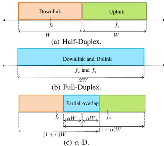
Fig. 1: An illustrative diagram showing  $\alpha$ -D scheme.
