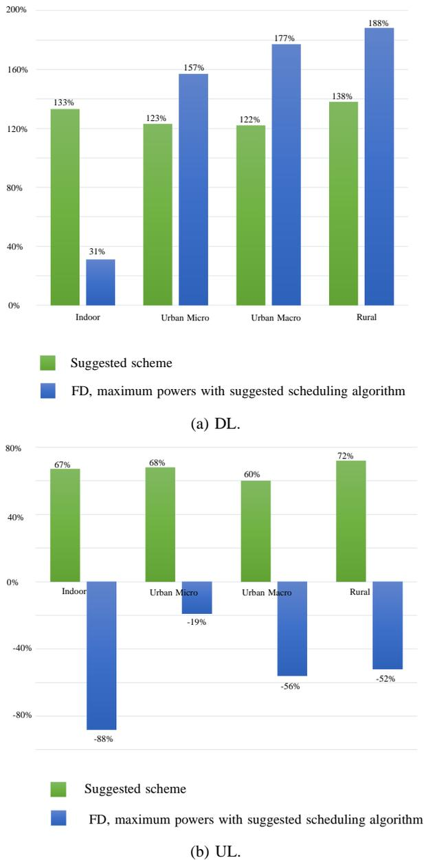
Fig. 10: Chart showing the gain from FD/ $\alpha$ -D compared to HD communication for different network environments, for sum of log-rate maximization ( $p_{\min}^{(b)}/p_{\max}^{(u)}=5$  dB).
