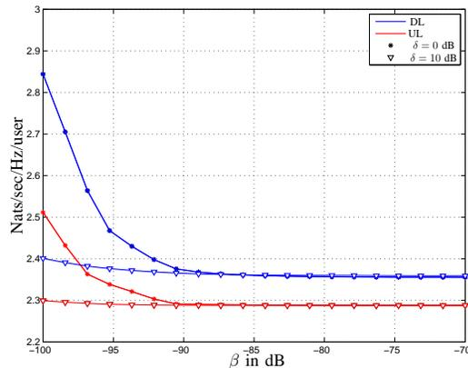
Fig. 8: Variation of the UL and DL rate according to the level of SIC in dB for different level of power disparity,  $B = 9$ ,  $K = 3$  for micro urban environment.
