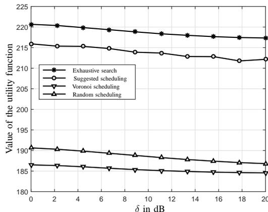
Fig. 5: Variation of the utility function for  $\alpha$ -D with optimized  $\alpha$  and power, using different scheduling algorithms,  $B = 2$ ,  $K = 3$  for micro urban environment.
