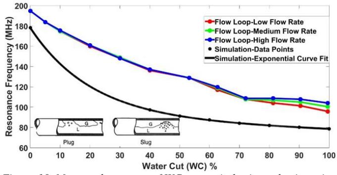
Figure 10. Measured response of WC sensor in horizontal orientation at three different flow rates along with simulated curve. Inset shows the Plug/Slug flow regime observed in horizontal tests section
