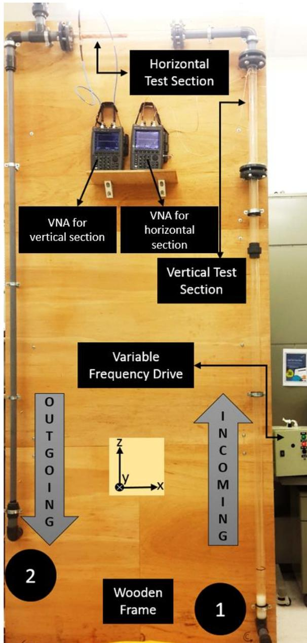
Figure 4. Front side of the flow loop (Main circulation piping on the wooden frame)
