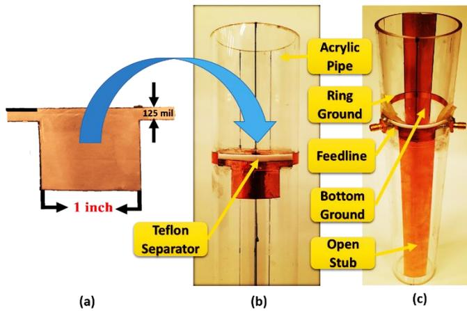
Figure 2. (a) Laser-cut feedline (and partial stub length) (b) acrylic pipe with teflon piece separating the feedline and its corresponding ring-ground (c) complete fabricated prototype with bottom ground plane, open stub and SMA connectors to characterize the sensor using Vector Network Analyzer
