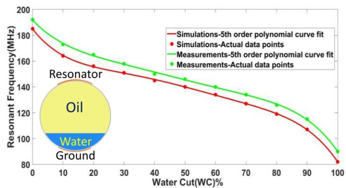
Figure 3. Simulated and measured responses of WC sensor. Inset picture shows the cross sectional view of pipe in this (static) characterization scenario
