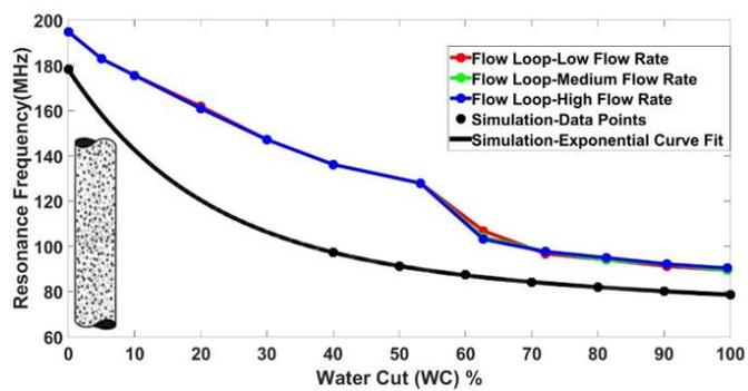
Figure 8. Measured response of WC sensor in vertical orientation at three different flow rates along with simulated curve. Inset shows the dispersed flow regime observed in vertical tests section
