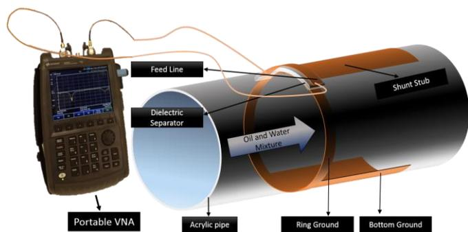
Figure 1. Pipe conformable T-resonator (used as WC sensor) along with portable VNA to extract its transmission coefficients
