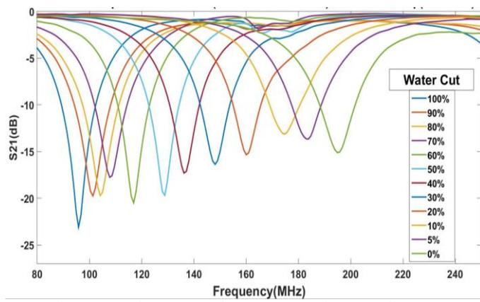
Figure 9. Measured response of WC sensor in horizontal orientation at low flow rate (40Hz freq. of VFD)
