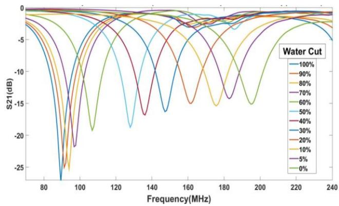
Figure 7. Measured response of WC sensor in vertical orientation at low flow rate (40Hz freq. of VFD)
