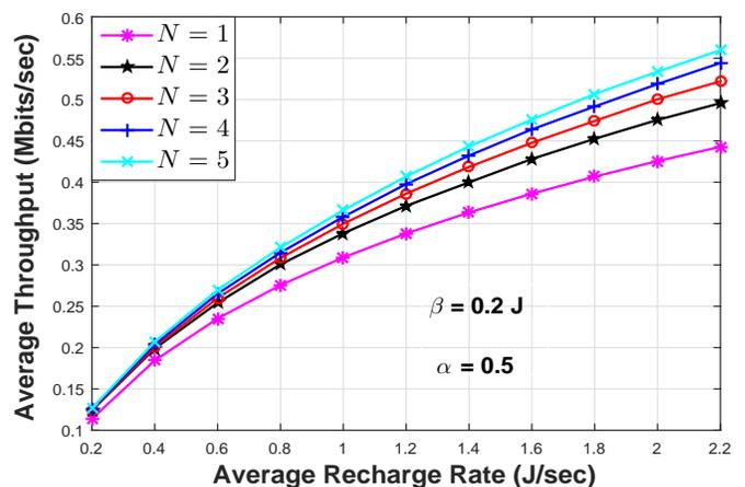
Fig. 6. Performance of the online policy with Rayleigh fading channels for various sensing periods,  $E_{max} = 100$  J and  $\sigma^2 = 1$ .
