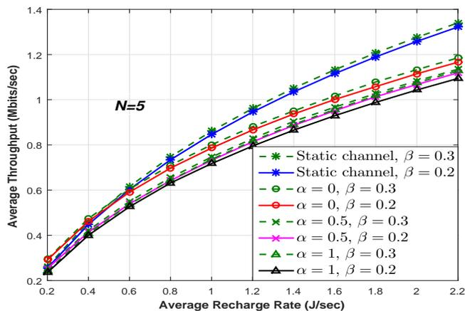
Fig. 4. Performance of the online policy with Rayleigh fading channels for various channel estimation errors,  $E_{max} = 100$  J and  $\sigma^2 = 1$ .
