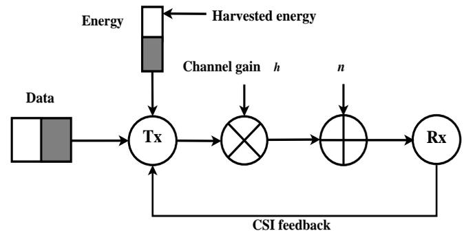
Fig. 1. An energy harvesting communication system model with CSI feedback.
