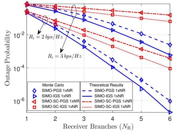
Fig. 7. Outage probability vs. number of receiver streams in HWD receive diversity system.
