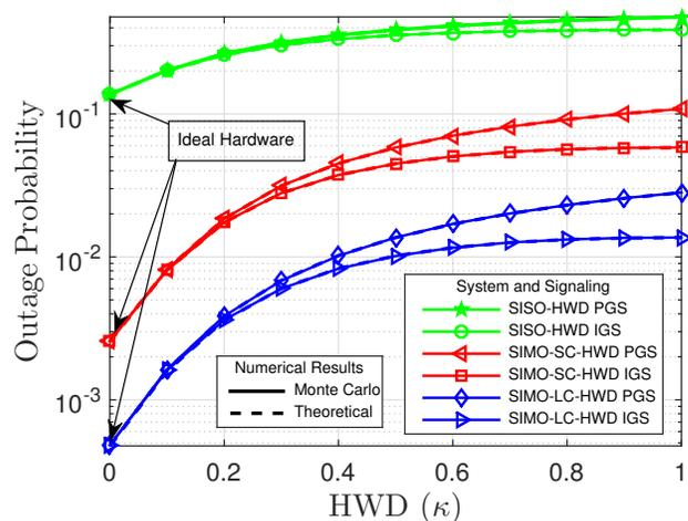
Fig. 3. Outage probability vs. HWD level in SISO and SIMO transceivers
