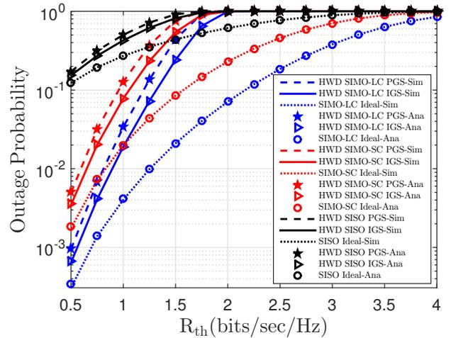
Fig. 6. Outage probability vs. target achievable rates
