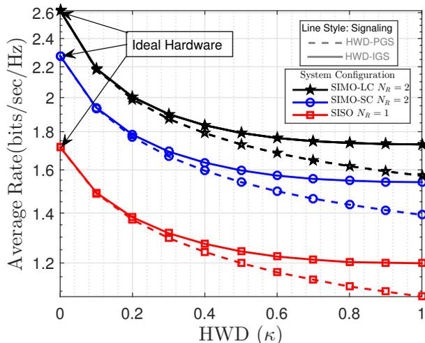
Fig. 2. Average achievable rate vs. HWI level in SISO and SIMO transceivers
