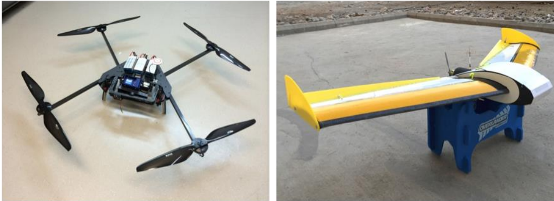
Figure 1. Quadcopter (left) and fixed-wing (right) UAV systems for precision agriculture. Each UAV has approximately 20+ minutes of flight time, making them suitable for reasonably large area coverage (10-50 Ha.), dependent on flying height.
