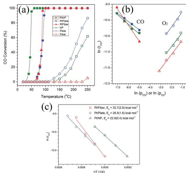
Fig. 3 (a) Catalytic activity of the Pt-loaded (solid) and Pt-free (open) PT nanocrystals (green), nanofibers (red) and nanoplates (blue); (b) reaction orders for CO (solid) and O<sub>2</sub> (open) of the three corresponding Pt/PT nanostructures and (c) Arrhenius plots and linear regression analysis.
